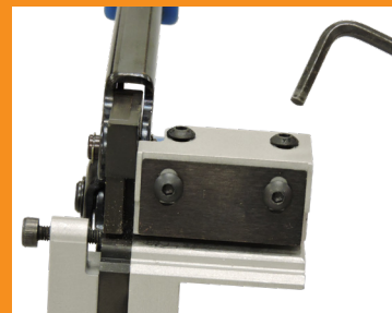
Adjust depth with the side block using horizontal screws
